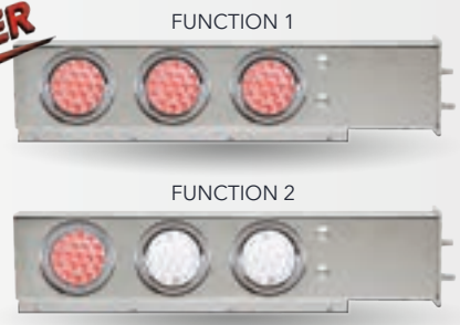
RED STOP, TURN & TAIL TO WHITE BACK UP TU-9210L2 Clear Lens
