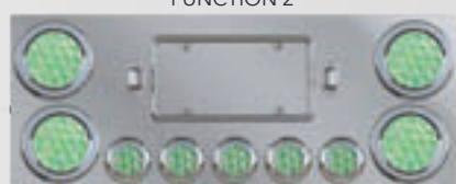
▲ RED STOP, TURN & TAIL TO GREEN AUXILIARY TU-9002L6 Clear Lens
