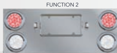
RED STOP, TURN & TAIL TO WHITE BACK UP TU-9017L4 Clear Lens
